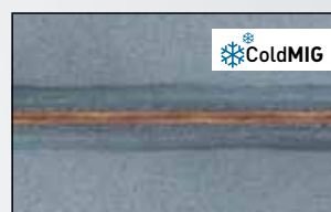
MIG brazing of galvanized sheet metals
